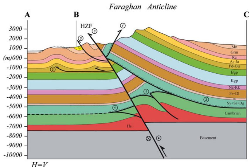
**Fig. 11** Structural cross-section through Kuh-e-Faraghan (see location on Fig. 3). *Hs* Late Proterozoic to Infra-Cambrian Hormuz Salt, *Sy* Ordovician Syahoo Fm. *Dg* Hirnantian Dargaz Fm., *Sr* Silurian Sarchahan Fm., *Zk* Devonian Zakeen Fm., *Fr* Early Permian Faraghan Fm., *Dl* Permian Dalan Fm., *Kk* Triassic Khanehkat Fm., *Nz* Jurassic Neyriz
