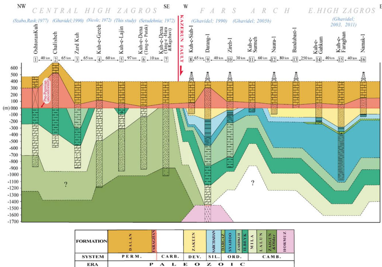
**Fig. 5** Stratigraphic correlation diagram of pre-Faraghan Palaeozoic formations in High Zagros Belt. Datum: base Faraghan formation. (See Fig. 1 for location of the columns). Note to the references of the surface
