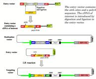
The destination vector contains the region homologous to the Dct gene, as well as the negative and positive selection cassettes. The LR reaction allows the insertion of the cDNA of interest within the destination vector though producing the largeting vector.
