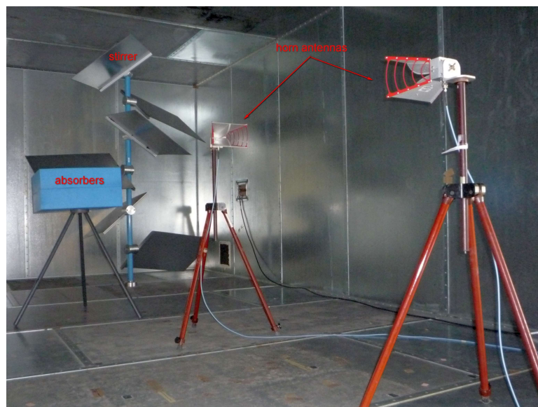
Figure 3.5: Reverberation chamber measurement configuration.
