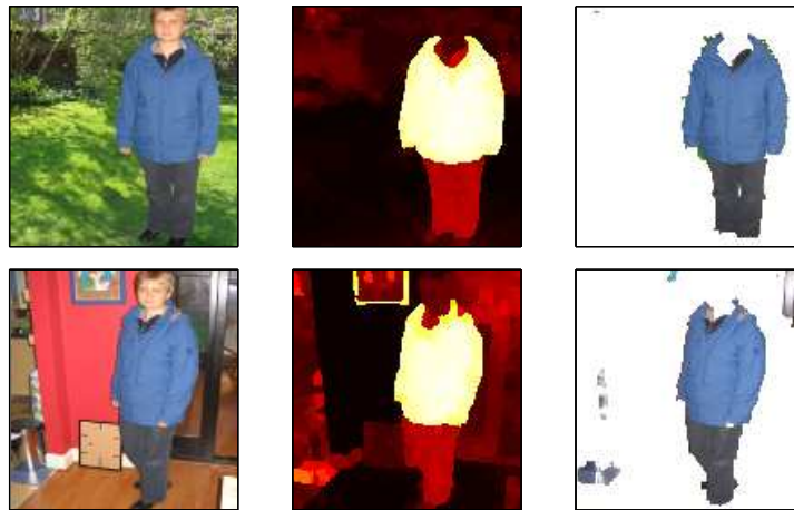
Figure 2.4: A failure case: (left) input images, (middle) scores obtained by our algorithm, (right) co-segmentation. We use \mu = 0.001 .
