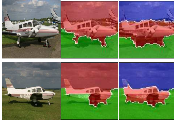
Figure 4.4: This figure shows how increasing the number of classes leads to a better segmentation. Columns 2 to 3 respectively show results for K = 2 and K = 3 (best seen in color).
