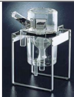
Figure 27: A representative picture of a metabolic cage allowing to house up to 5 mice. Mice are placed on a grid. Urine and feces fall across the grid and are separated thanks to a funnel.
