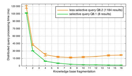
Figure 8.1: Decreasing distributed query processing (DQP) time for a large scale knowledge base (1.7M triples) fragmented through up to 16 data stores, under *full* query rewriting strategy.
