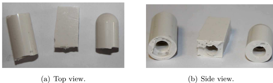
FIGURE 6.4 – Silicone fingertips of three different shapes : B-C-A
