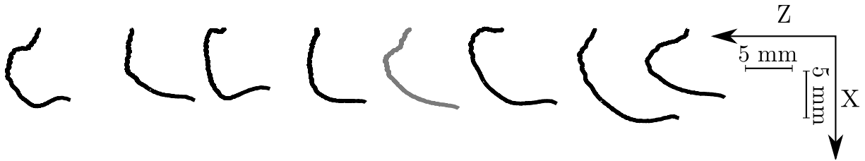
FIGURE 6.6 – Harpist forefinger movement during plucking actions. The grayed movement is used as reference for the robot.
