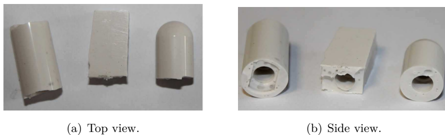
FIGURE 6.4 – Silicone fingertips of three different shapes: B-C-A
