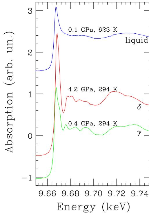
Figure 7.13: XANES spectra of the three observed phases of  $\text{ZnCl}_2$ . Large variations in the  $4p$  density of states above the Fermi level can be observed between  $\gamma$ - $\text{ZnCl}_2$  and  $\delta$ - $\text{ZnCl}_2$ .
