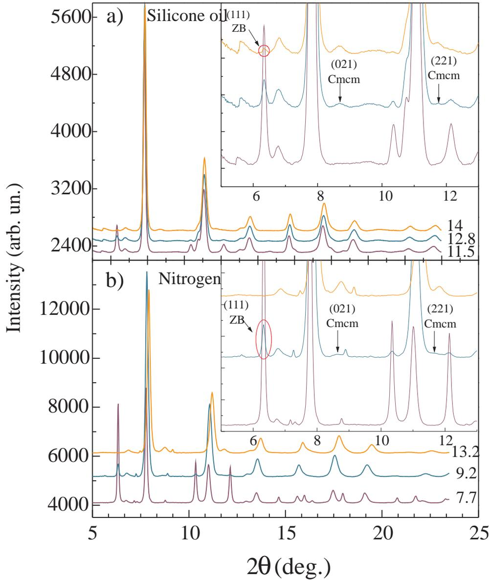
Figure 8.17: a) Transition from NaCl to *Cmc m* in the data recorded using Silicone oil as PTM. The inset shows the appearance of the (021) and (221) peaks of *Cmc m* at 12.8(7) GPa and the (111) reflection of ZB at 14(1) GPa. b) Transition from NaCl to *Cmc m* in the data recorded using Nitrogen as PTM. The inset shows at 9.2(1) GPa the co-existence of reflections attributed to the ZB and *Cmc m* phases.
