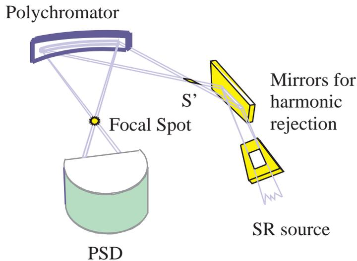
Figure 6.1: Scheme of the dispersive XAS concept.
