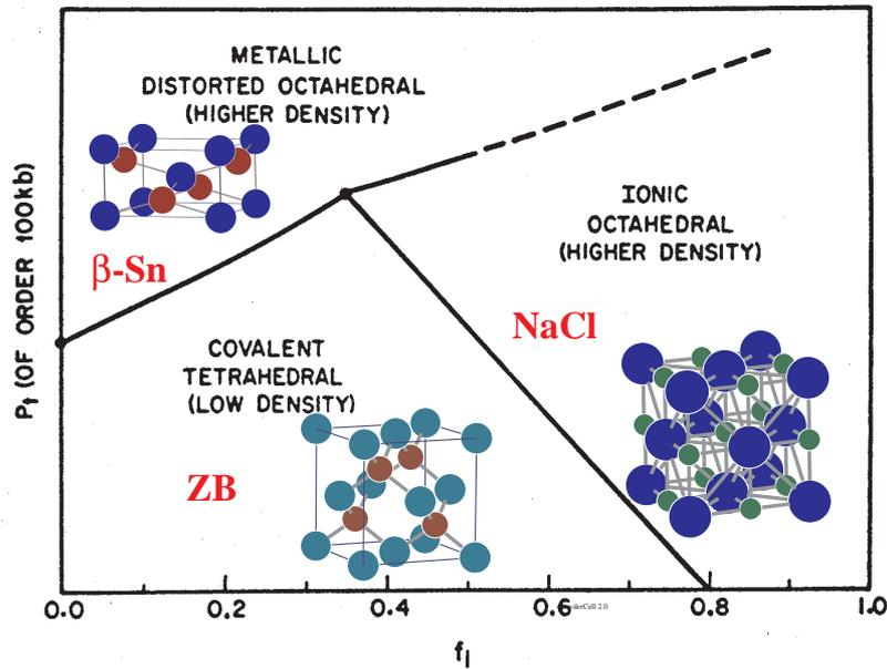
Figure 8.9: Schematic ( $f_i$ ,  $P$ ) phase diagram showing the covalent, ionic, and metallic structures of  $A^N B^{(8-N)}$  compounds.
