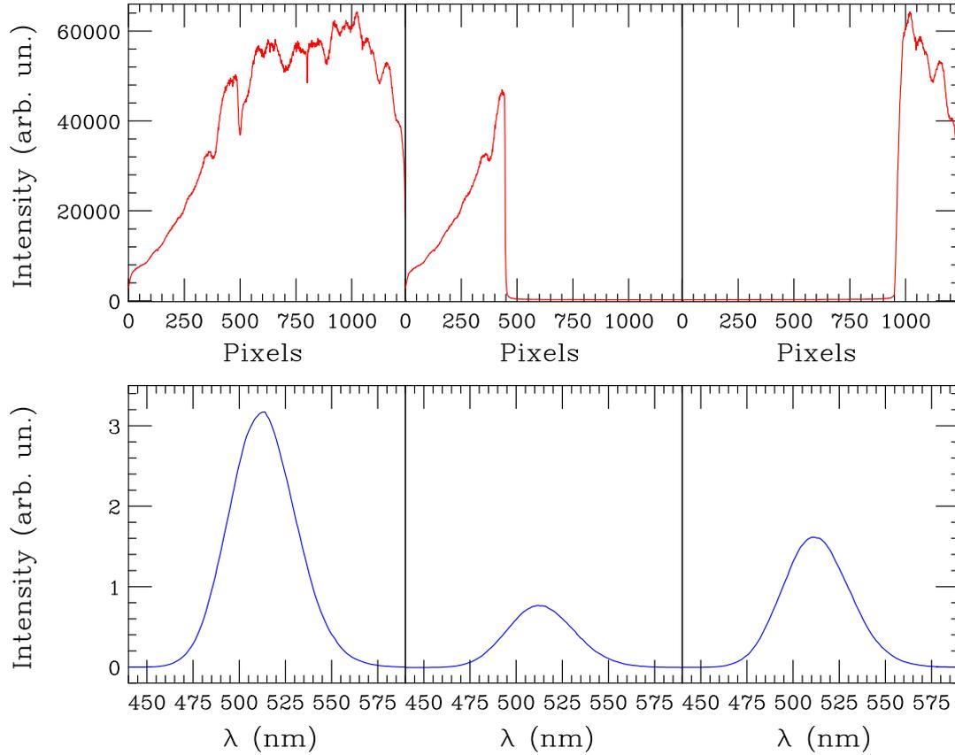
Figure 3.19: The three *upper panels* show the total polychromatic beam diffracted by the crystal in the energy range 11.400 - 11.990 keV (*left*), the beam below (*middle*), and above (*right*) the Pt  $L_3$ -edge, respectively. The three *lower panels* show the corresponding emission spectra.
