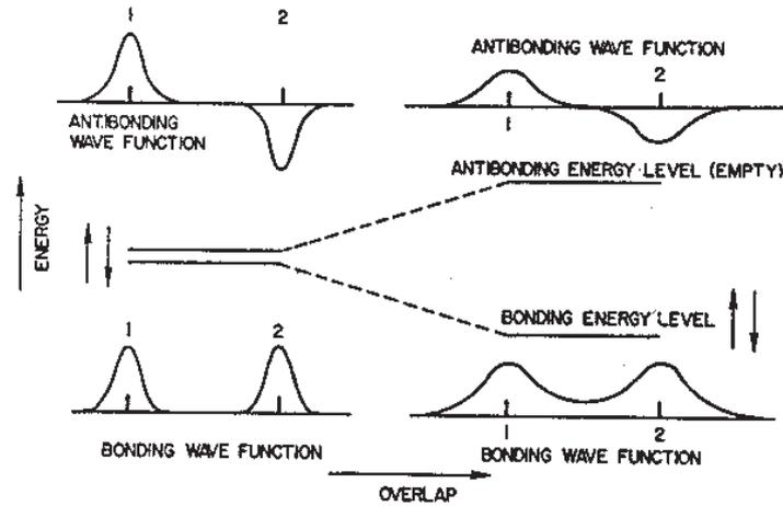
Figure 8.1: Formation of bonding and antibonding states on going from atom to crystal. In bonding states the wave function amplitude  $\psi_b$  associated with a directed orbital centered on atom 1 interferes constructively or in phase with a similar orbital centered on atom 2 in the bonding region between atoms 1 and 2. Similarly, the amplitude  $\psi_a$  of the antibonding orbital exhibits a node in the bonding region.
