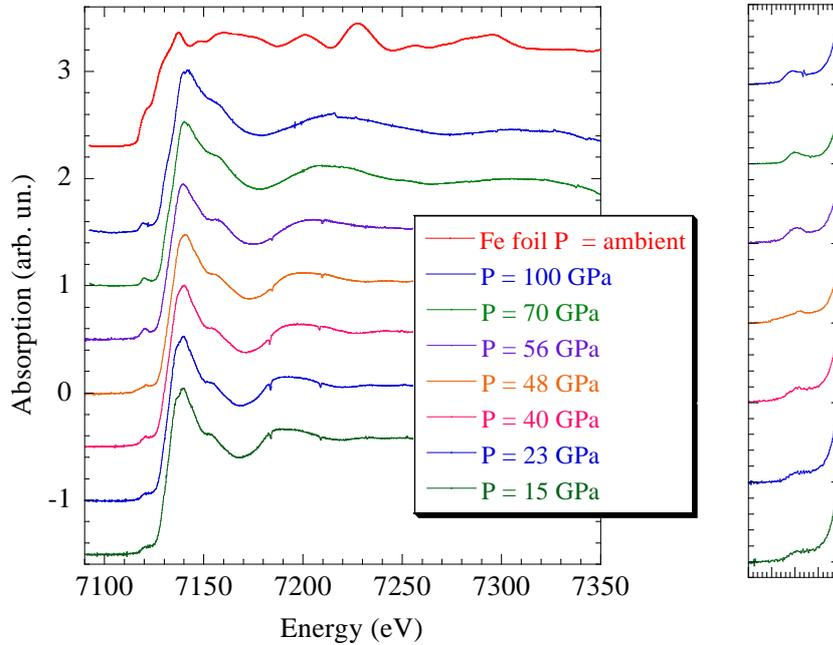
Figure 7.8: First HP XAS on hematite  $\text{Fe}_2\text{O}_3$  up to 100 GPa (*left panel*). Modifications of the pre-edge features and of the shape of the absorption edge are clearly detectable as a function of pressure (*right panel*).
