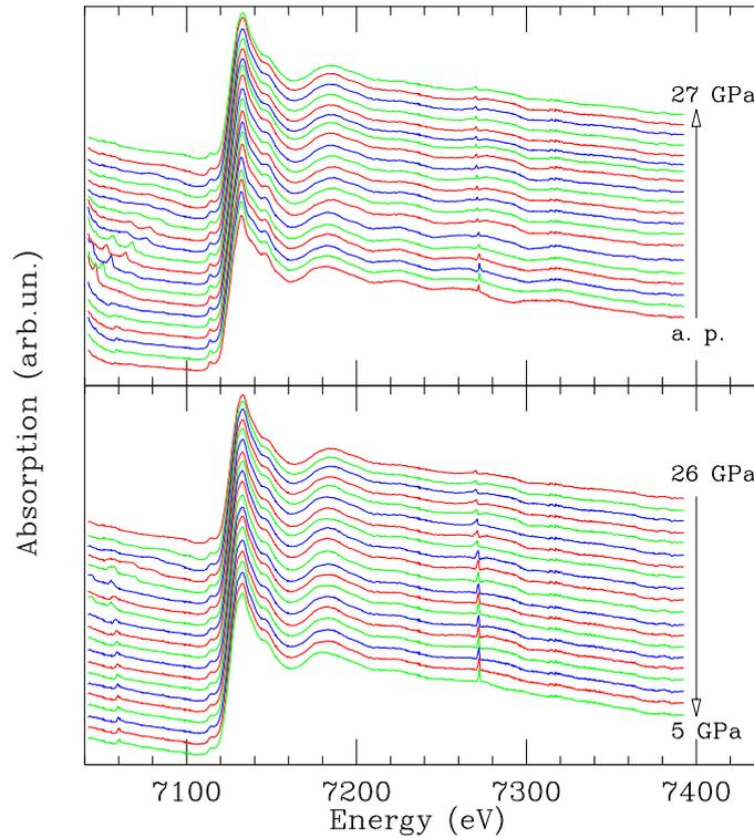
Figure 7.6: XAS spectra of  $\gamma$ -Fe<sub>2</sub>O<sub>3</sub> from ambient pressure up to 27 GPa (*upper panel*) and from 26 GPa down to 5 GPa (*lower panel*).
