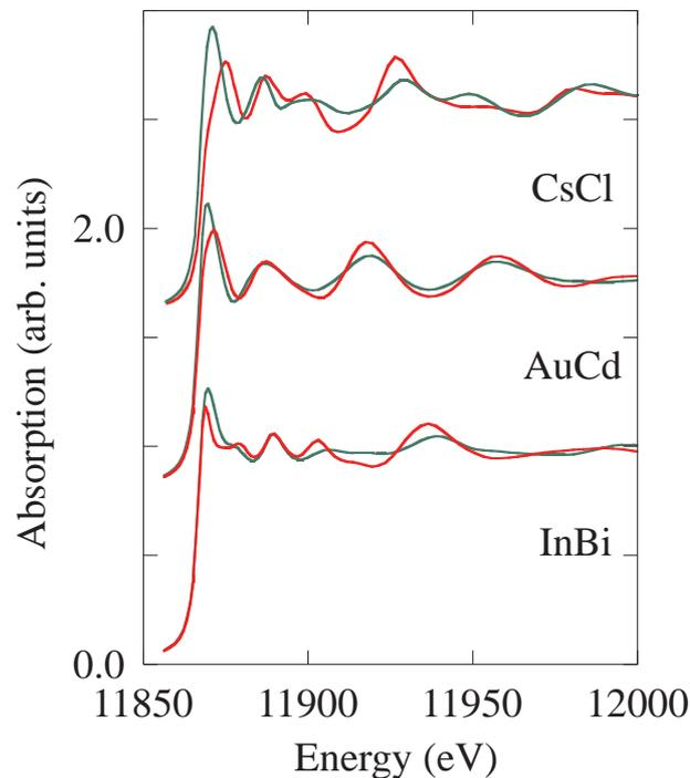
Figure 8.29: Simulated spectra based on the proposed HP phases for InAs: CsCl, AuCd and InBi. Green/red lines correspond to chemically-disordered/ordered clusters respectively.
