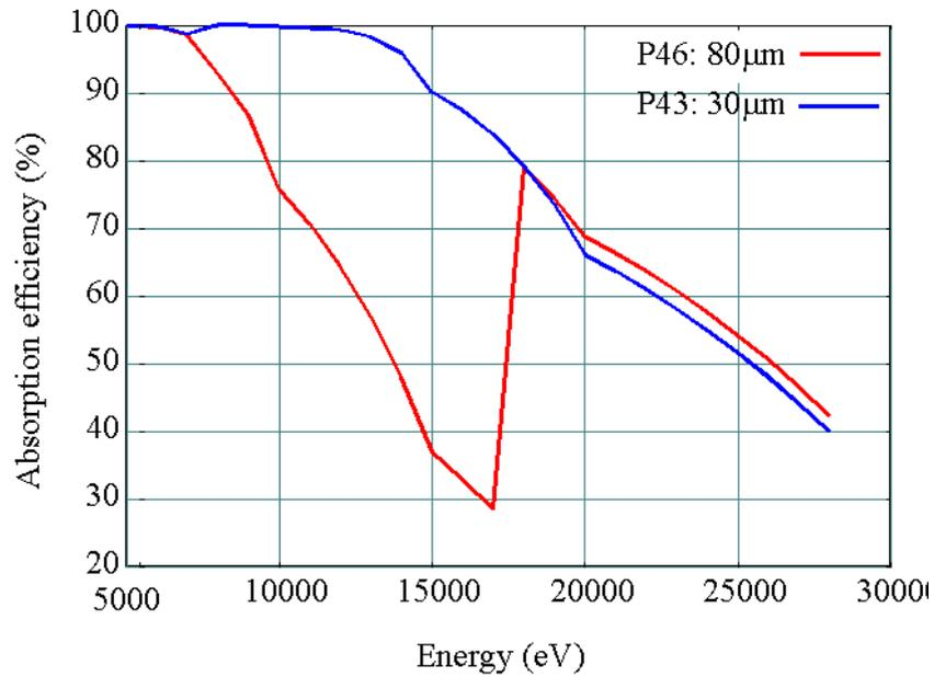
Figure 2.2: Absorption efficiency as a function of energy.
