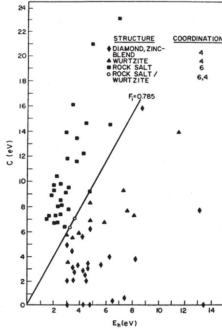
Figure 8.4: Values of  $E_h$  and  $C$  for crystals of the type  $A^N B^{(8-N)}$ . The coordination numbers are indicated. Note that  $F_i = 0.785$  separates all four-fold from all six-fold coordinated crystals.
