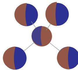
Figure 8.11: Drawing of a possible configuration of site-disordered InAs in the zincblende structure.
