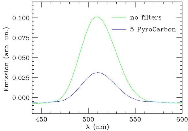
Figure 3.18: Emission band of  $\text{Pt}_2(\text{P}_2\text{O}_5\text{H}_2)_4^{4-}$  under excitation with X-rays not attenuated by filters (*green line*), and attenuated by 5 mm of Pyrocarbon (density: 2.26  $\text{gr}/\text{cm}^3$ ) (*blue line*).
