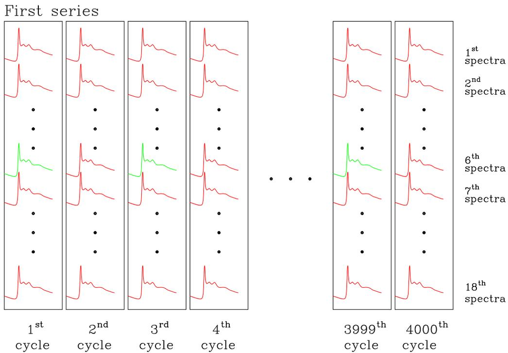
Figure 3.9: The acquisition strategy of the first series: the laser is fired at each 6<sup>st</sup> spectrum of every odd cycle (green spectrum).
