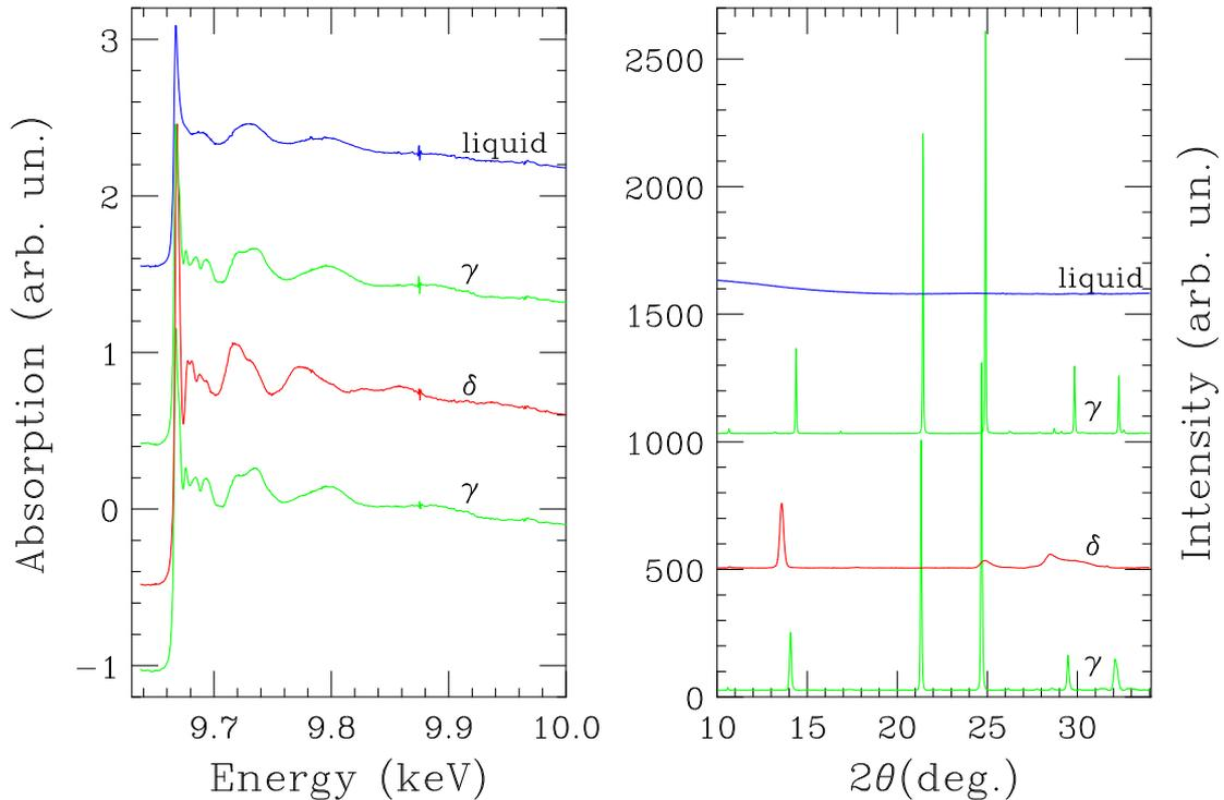
Figure 7.12: XAS spectra of  $\text{ZnCl}_2$  at different pressure and temperature conditions and relative XRD patterns at the same conditions.
