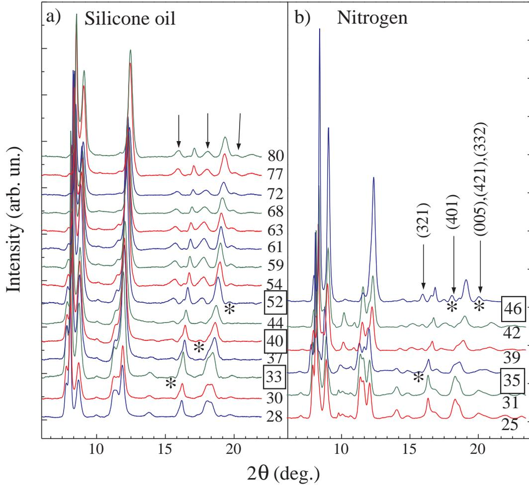
Figure 8.18: Transition from *Cmc* to *Pmma* in the data collected using Silicone oil (*left panel*) and Nitrogen (*right panel*) as PTM. The arrows indicate the new reflections forbidden by the C-centering condition of the *Cmc* space-group. In the data recorded using Nitrogen the new peaks are indexed. The stars indicate the appearance of the new *Pmma* peaks.
