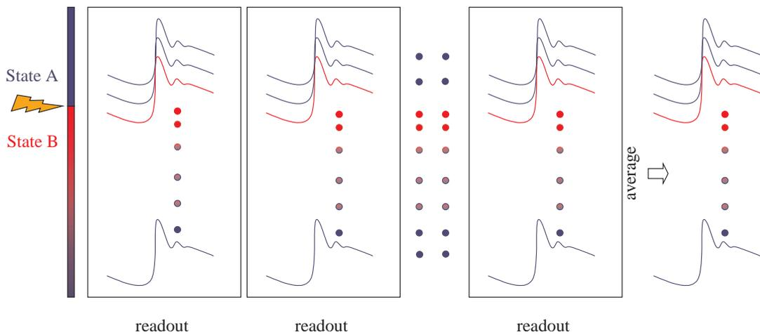
Figure 2.5: Fast acquisition method: the corresponding spectra of different cycles are averaged.
