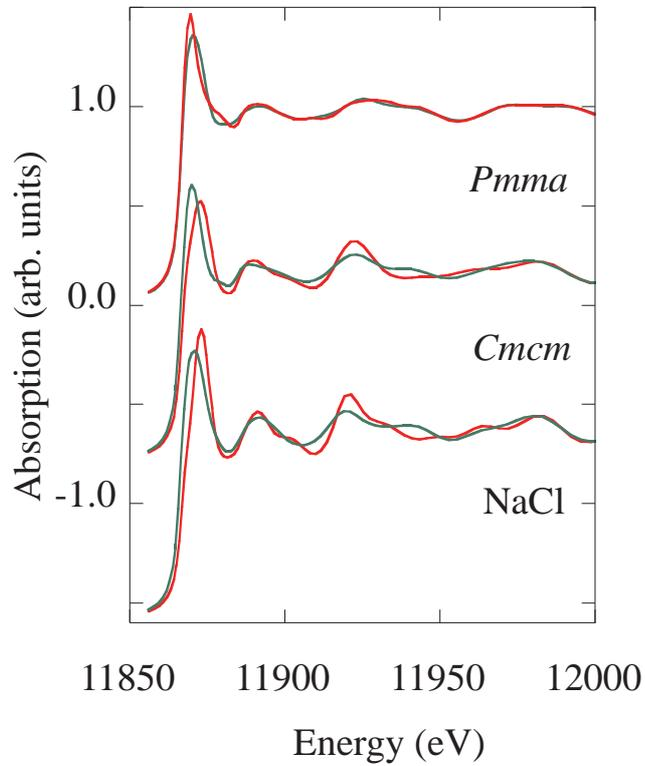
Figure 8.30: Simulated spectra of short-range chemically-ordered/disordered (*red/green lines*): NaCl at 15 GPa, *Cmcm* at 25 GPa, and *Pmma* at 40 GPa.
