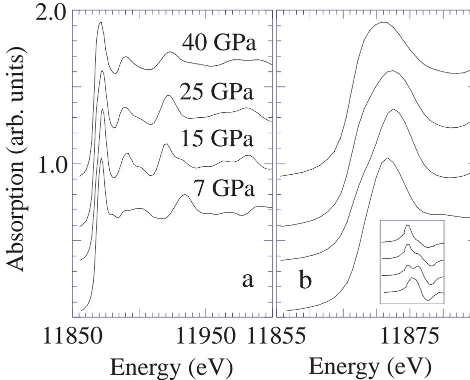
Figure 8.31: a) Simulations that best correspond to the data shown in Figure 8.24: ZB at 7 GPa, short-range chemically-ordered NaCl at 15 GPa, short-range chemically-ordered  $Cmcm$  at 25 GPa and 50% linear combination of short-range chemically-ordered  $Cmcm$  and short-range chemically-disordered  $Pmma$  at 40 GPa. b) Edge region: the inset shows the trend on the derivatives.
