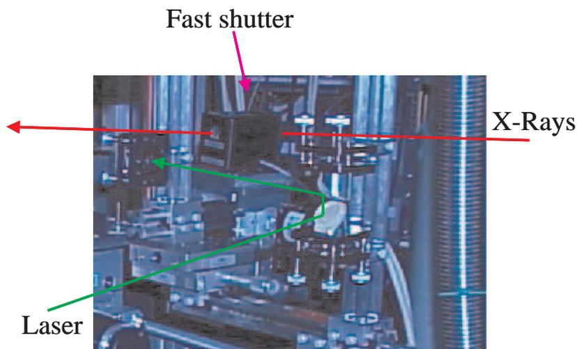
Figure 3.6: The laser beam, initially parallel to the X-ray beam is reflected in the vertical direction by a high-energy  $45^\circ$  incidence beam-steering mirror for UV-light, the beam is then reflected by a second mirror and focused by concave lens onto the sample.
