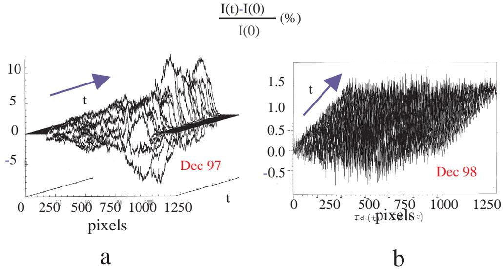
Figure B.2: Relative intensity variations  $[I(t)-I(0)]/I(0)$  measured on the CCD detector as a function of time: a) before and b) after installation of the local feedback.
