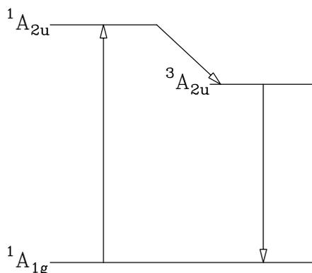
Figure 3.2: Energy level diagram of the lowest excited state of  $\text{Pt}_2(\text{P}_2\text{O}_5\text{H}_2)_4^{4-}$  under  $D_{4h}$  symmetry.
