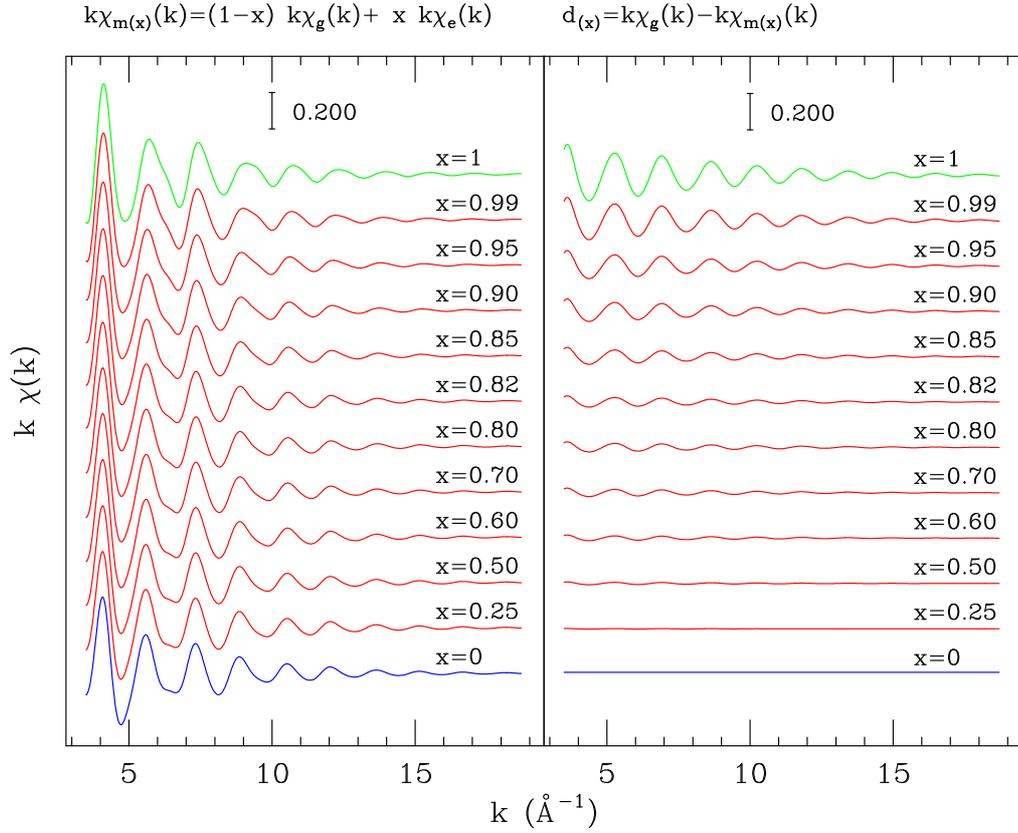
Figure 3.12: *Left panel*: different linear combinations  $k\chi_{m(x)}(k)$  of the best-fit XAFS signal  $k\chi_g(k)$  and the simulated XAFS signal  $k\chi_e(k)$ . From bottom to top, the  $k\chi_{m(x)}(k)$  functions have an increasing weight of the  $k\chi_e(k)$  term. *Right panel*: difference between  $k\chi_g(k)$  and  $k\chi_{m(x)}(k)$  with an increasing value of  $x$  from bottom to top.
