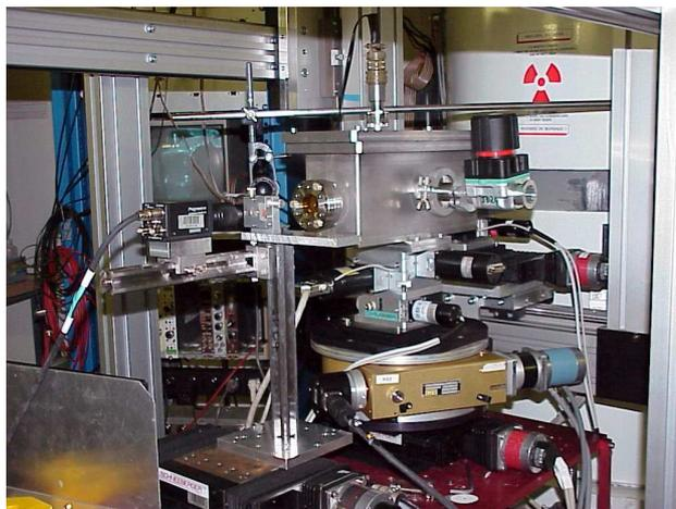
Figure 7.2: The vacuum chamber of the third refocusing mirror. The chamber is installed downstream the polychromator, at about 0.5 m from the sample.
