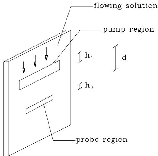
Figure 3.3: Schematic view of the sample holder. By varying  $d$ , the displacement between the laser beam and the X-ray beam, one can monitor the kinetics of the decay of the excited state. This parameter  $d$  provides the time delay  $\Delta t$  given as  $\Delta t = d/v$  where  $v$  is the velocity of the flowing sample.
