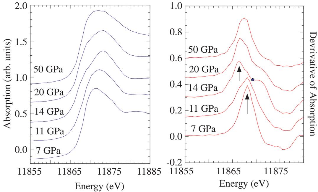
Figure 8.26: *Left panel*: edge region of the spectra. *Right panel*: derivative with respect to the energy. The blue dot indicates a discontinuity in the first derivative of the metallic phase. The arrows indicate a shift of the absorption edge from the semiconducting to the metallic phase.
