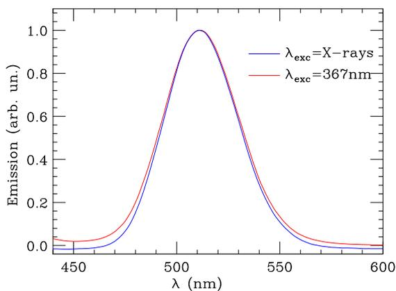
Figure 3.17: Emission band of  $\text{Pt}_2(\text{P}_2\text{O}_5\text{H}_2)_4^{4-}$  under excitation with X-rays (*blue line*), and 367 nm (*red line*). The two emission bands are normalized to the maximum of the intensity to show that they correspond to the same transition  ${}^3A_{2u} \rightarrow {}^1A_{1g}$ .
