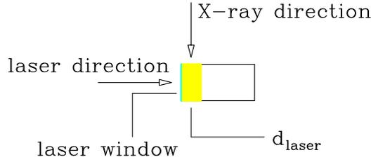
Figure 3.4: Geometry in which the laser beam and the X-ray beam are perpendicular to each other.
