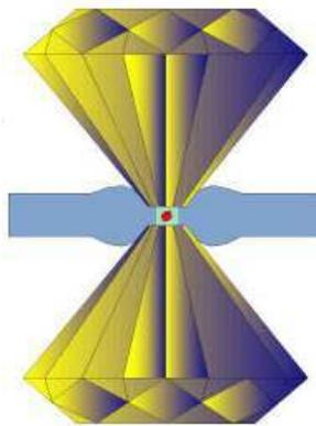
Figure 5.2: The principle of the diamond anvil cell.
