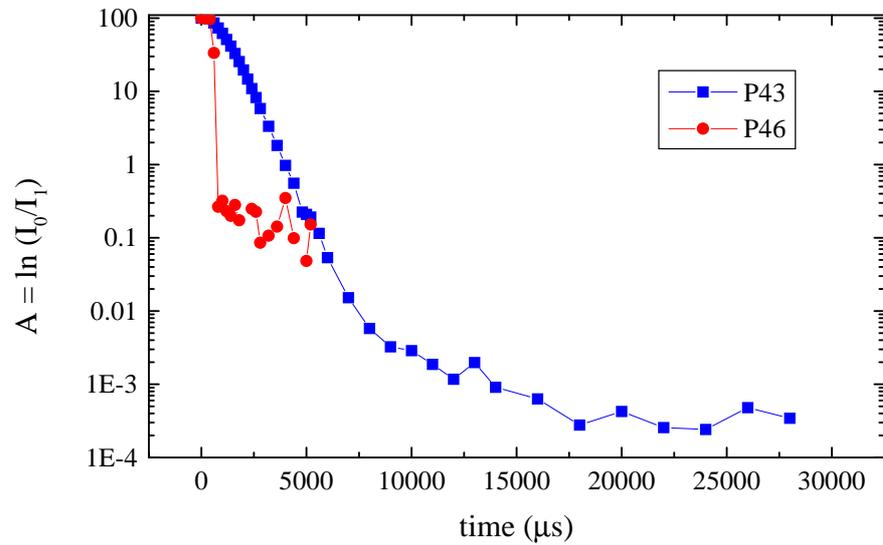
Figure 2.3: Measured temporal response: the shutter is closed at  $t = t_0 = 400 \mu s$ .
