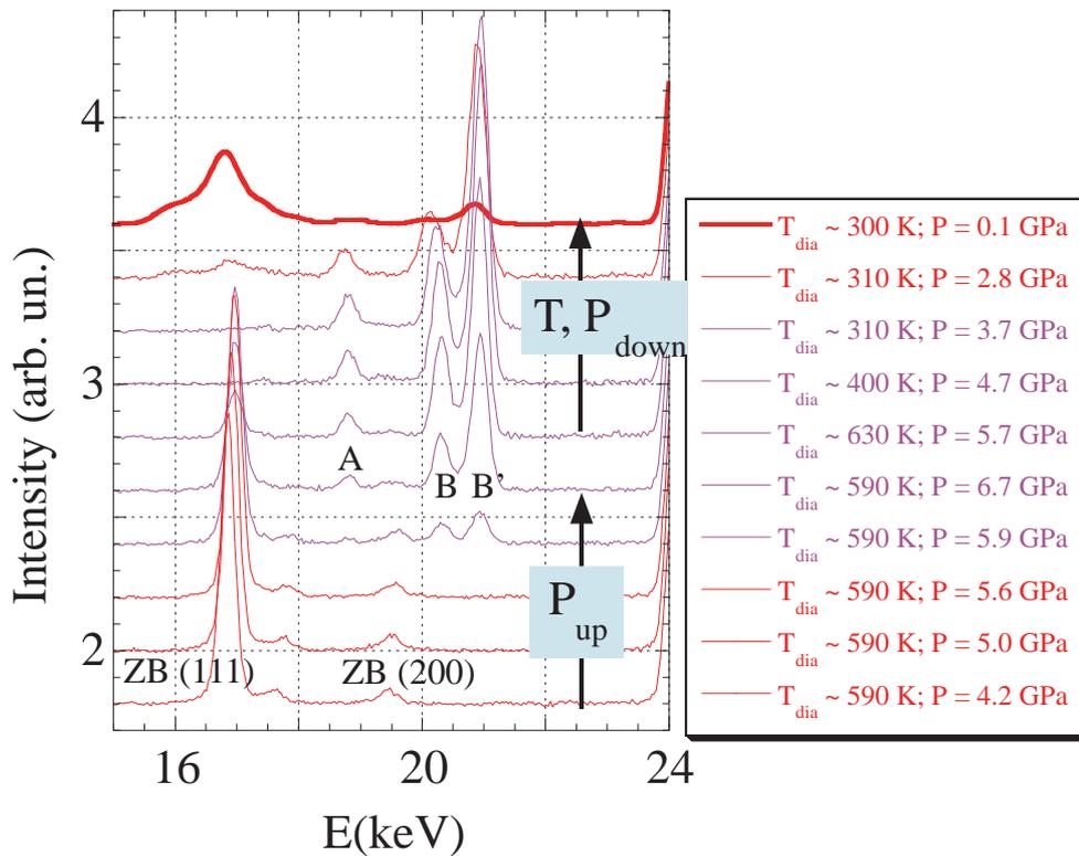
Figure 8.35: Some of the profiles relative to Run 4. At  $T_{dia} \sim 590$  K, we clearly observe the onset of features A, B and B' at  $P \sim 5.9$  GPa. On temperature and pressure release, these peaks persist with the same intensity down to about RT and  $P < 3$  GPa. At this pressure, very wide ZB reflections appear. At ambient condition (in bold) peaks B and B', although very weak and large, are still detectable.
