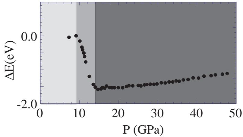
Figure 8.27:  $\Delta E$  as a function of pressure. The evolution of  $\Delta E$  with pressure can be used to identify three distinct pressure regions in which the electronic properties of InAs differ:  $P < 9$  GPa (*light grey*) semiconducting InAs,  $9$  GPa  $< P < 14$  GPa (*medium grey*) coexistence of semiconducting and metallic InAs,  $P > 14$  GPa (*dark grey*) metallic InAs.
