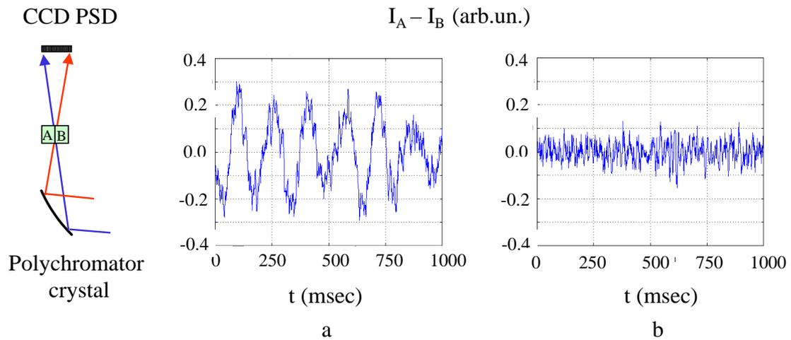
Figure B.3: Time evolution of the current difference  $I_A - I_B$  from fast PIN photodiodes A and B positioned just in front of the sample, as shown on the left of the figure. a) before and b) after activation of the local horizontal feedback.
