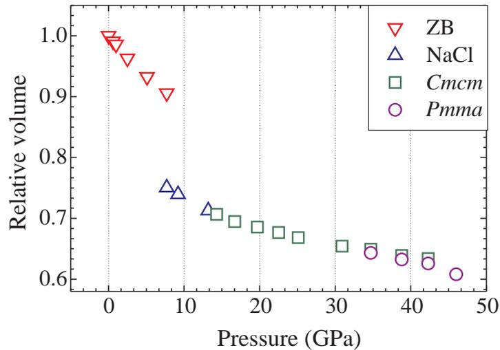
Figure 8.19: Relative volume of InAs versus pressure for Nitrogen data. A change in volume of  $\sim 18\%$  is associated to the ZB  $\rightarrow$  NaCl transition. No obvious volume discontinuities are observed in the other phase transitions.
