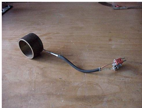
Figure 5.4: External heater for Chervin-type cell.
