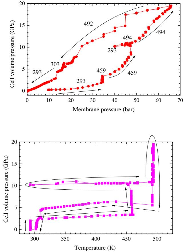
Figure 7.16: Pressure in the cell volume as a function of membrane pressure (*upper panel*) and the pressure in the cell volume for different values of temperature on the diamond (*lower panel*).
