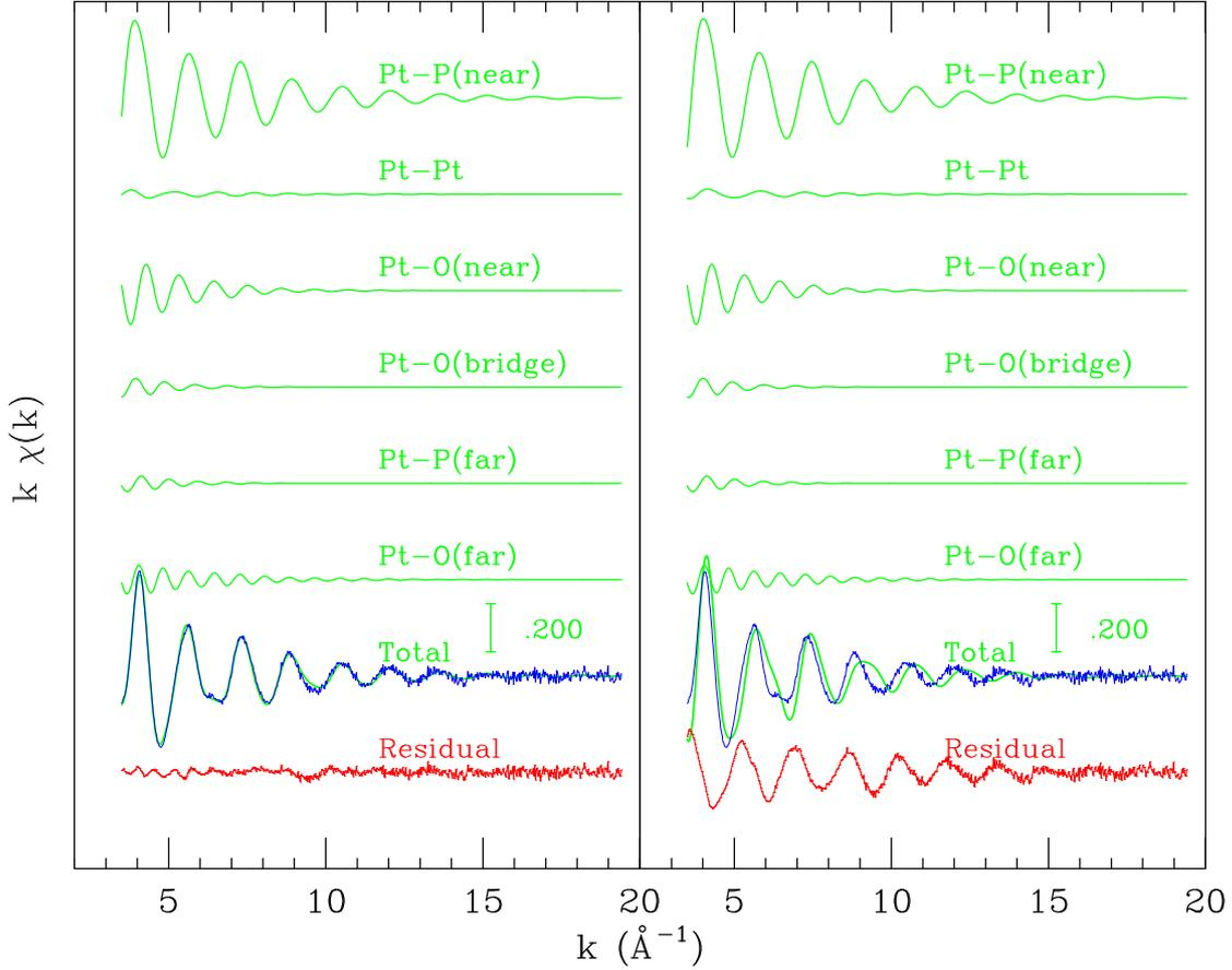
Figure 3.11: *Left Panel*: comparison of experimental and calculated best fit  $k\chi(k)$  XAFS signal of  $\text{Pt}_2(\text{P}_2\text{O}_5\text{H}_2)_4^{4-}$ . *Right panel*: simulated XAFS signals of the triplet excited state of  $\text{Pt}_2(\text{P}_2\text{O}_5\text{H}_2)_4^{4-}$ .
