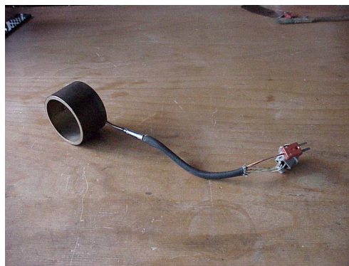
Figure 5.4: External heater for Chervin-type cell.
