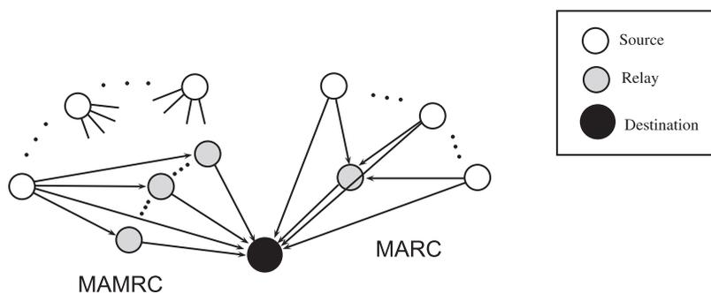
Figure 1.1: A multiple access relay channel (MARC) and a multiple access multiple relay channel (MAMRC)
