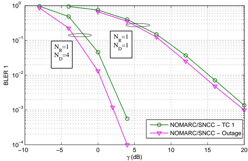
Figure 3.13: Individual BLER (e.g., for  $S_1$ ) - Practical NOMARC/SNCC vs. outage limit -  $\eta = 4/3$  b./c.u. - constellation expansion at the relay
