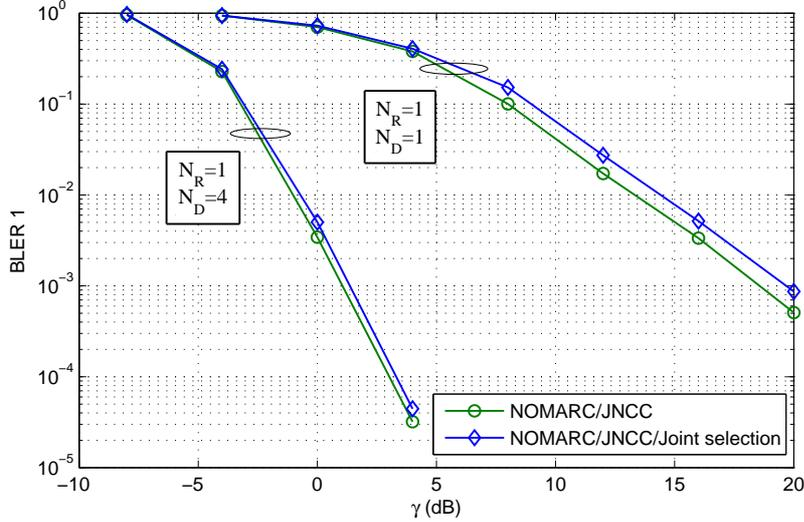
Figure 3.14: Individual BLER (e.g., for  $S_1$ ) - NOMARC/JNCC vs. NOMARC/JNCC/Joint selection -  $\eta = 4/3$  b./c.u.
