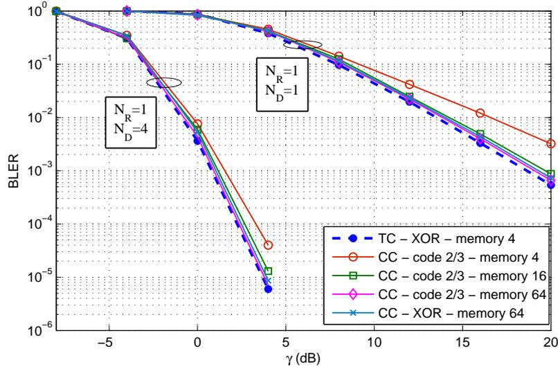
Figure 2.12: Joint BLER performance - error-free S-R links - Convolutional Code (CC) and Turbo Code (TC) at sources - JNCC based on XOR vs. JNCC based on double input binary linear code -  $\eta = 4/3$  b./c.u.
