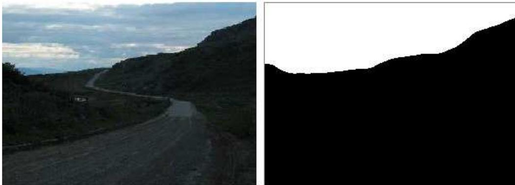
Figure 3.1 – Original image and Otsu segmentation.
