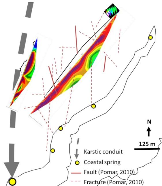
Figure 4- 39 : **Figure 5:** Location of ERT profiles, karstic conduit, fractures in the quarry and coastal springs. A connection exists between major fractures, electrical resistivity anomalies and secondary springs along the coast of Port-Miou.
