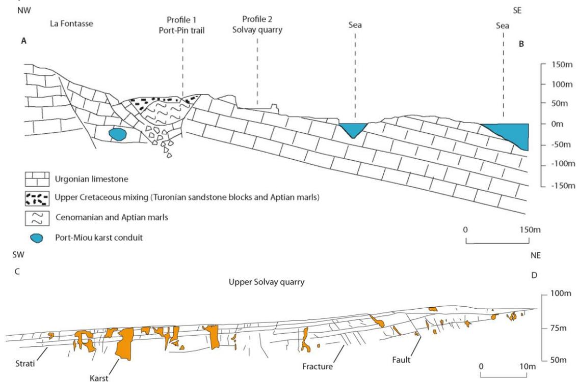
**Figure 4- 36 : Figure 2: Geological sections of the experimental site. Section AB is NW-SE and crosses the karstic conduit and profiles 1 and 2. A probable karstic collapse with marly limestone fillings is located above the conduit. Section CD is SW-NE and represents the upper wall of the Solvay quarry, showing dense fracturation and karstification in the urgonian limestones.**
