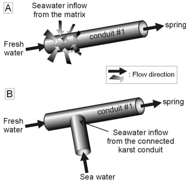
Figure 4- 26 : Fig.3 Conceptual model of seawater intrusion in a karst conduit feeding a brackish coastal spring. A diffuse saline intrusion by matrix-conduit exchange, B concentrate saline intrusion by connection of conduits.
