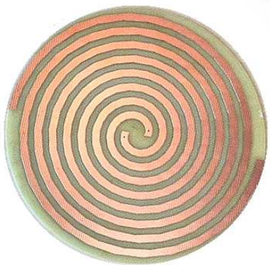
(a) Hardware model of spiral antenna over FR4 substrate
