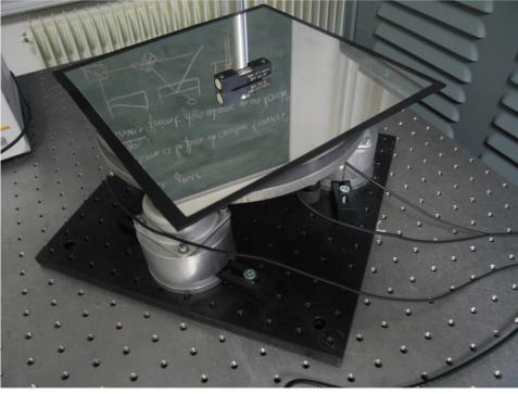
FIG. 6: The free-vibration active platform
