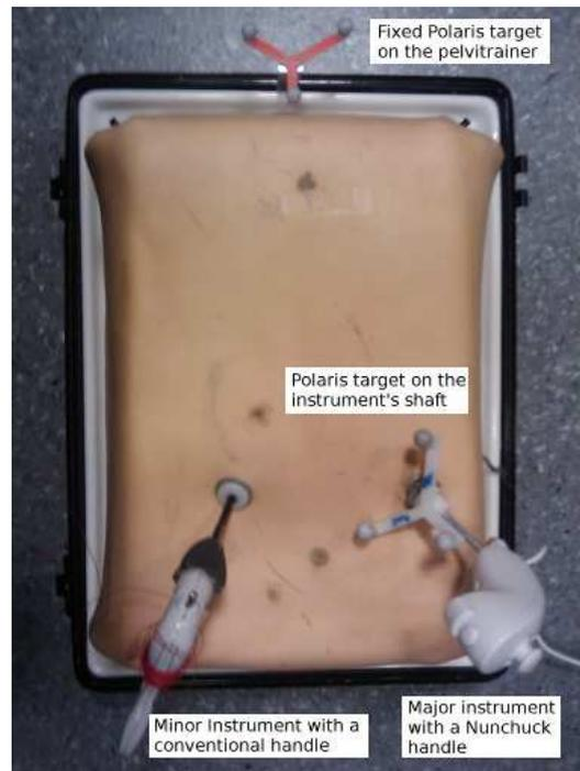
Figure 2.5: Pelvitrainer, 2 instruments and their Polaris targets
