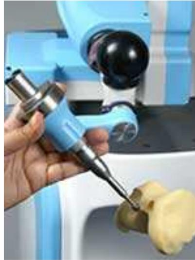
Figure 5: Acrobot<sup>®</sup>, a Parallel Comanipulation System for Orthopedic Surgery
