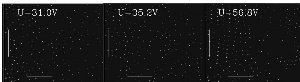
Figure 6.1: Phase transition as it occurs for increasing AC fields applied to a particle system levitated in PK-3 Plus [95].
