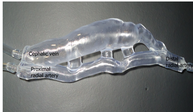
Figure 2.18: Phantom of the AVF: the 3-dimensional mould is obtained by rapid prototyping.
