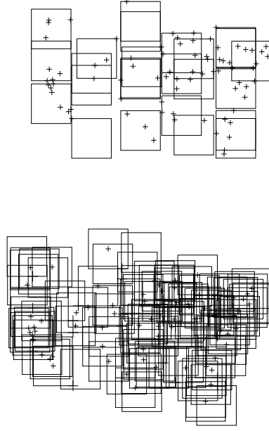
FIG. 2.4 – Finding a covering of 120 cities of the U.S.A. Our algorithm reports a set of 25 unit squares covering the 120 cities. Any solution requires at least 11 squares. (Considering the corresponding piercing problem, one may find 11 disjoint squares.)
