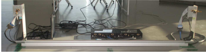
Fig. 5.11: Photograph of the setup with the radar system with a standard gain horn as antenna.
