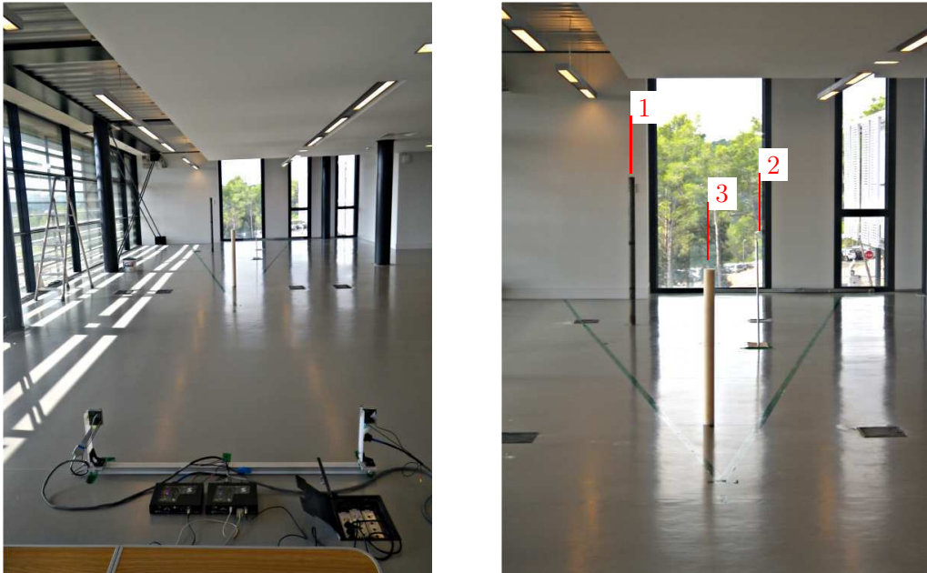
Fig. 5.14: Photograph of a three cylinders arrangement inside. Setup of the radar system with a standard gain horn as antenna (left). Scene of the three cylinders (right).
