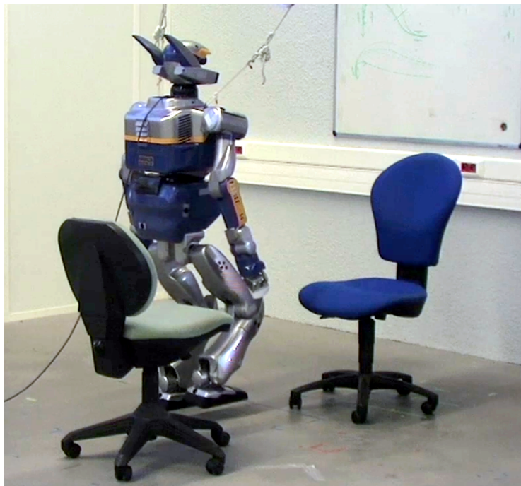
Figure 1.13: Humanoid Robot HRP-2 uses holonomic motion, or side-stepping, to pass between two chairs.
