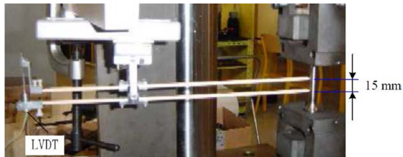
Fig. 4.2 Extensometer with 15mm distance between two sticks
