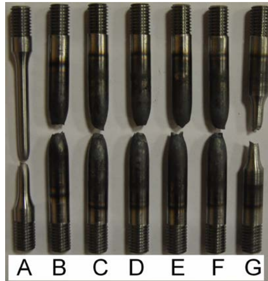
Fig. 5.26 Round bar samples after rupture
