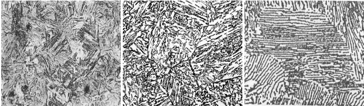
Fig. 2.9 Typical metallographics of martensite (left), bainite (middle) and pearlite (right)
