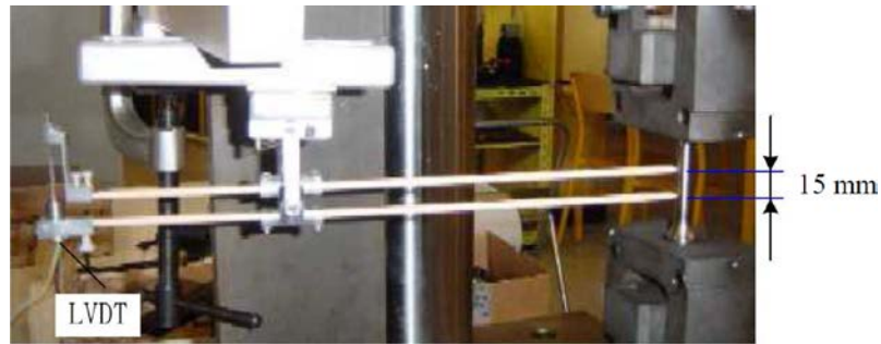
Fig. 4.2 Extensometer with 15mm distance between two sticks
