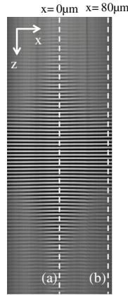
Fig. 3. (x, z) OCT intensity measurement in the plane y = 0 . Line (a) marks position x = 0 \mu\text{m} [profile shown Fig. 4(a)]. Line (b) marks position x = 80 \mu\text{m} [profile shown in Fig. 4(b)].
