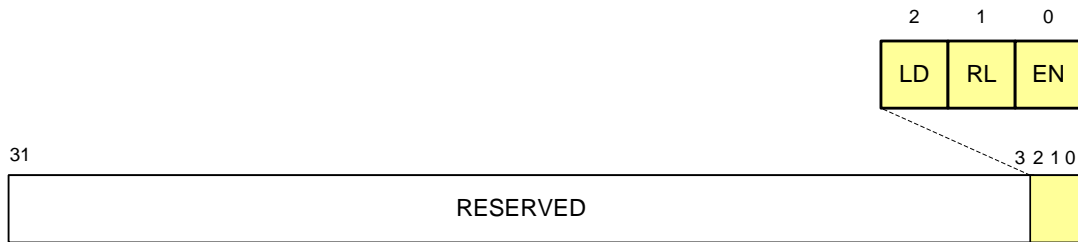
Figure 7.15: Timer Control Register.
