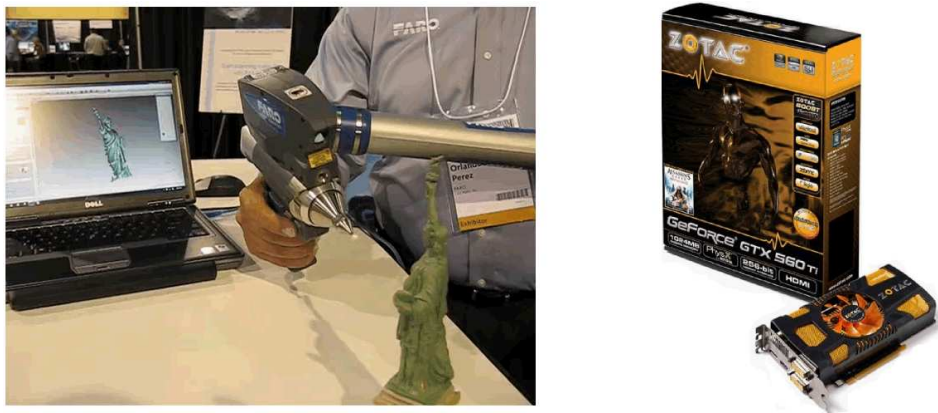
Figure 1.1 – 3D scanner (©Faro) and GeForce 3D accelerated graphic card (©NVIDIA).
