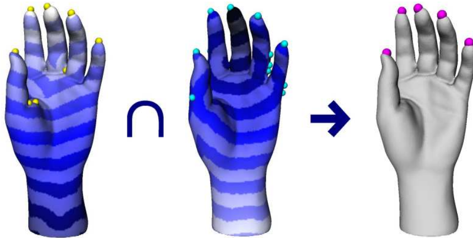
Figure 3.1 – The intersection of the two sets computed eliminates the unwanted feature points on a triangulated surface. (Figure taken from Tierny et al.(109))
