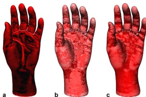
Fig. 11a–c. Several curvature estimations on the hand model: mean curvature (a), Gaussian curvature (b) and curvature index (c) [19]. The curvature index generates a more important contrast between convex and concave areas
