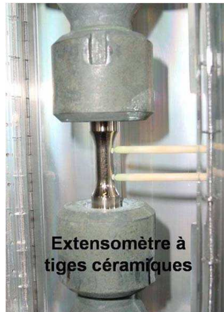
Figure 7 □ High temperature strain gage extensometer [1].
