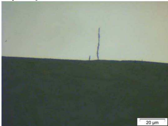
Figure 14 □ Cross section of 1630 MHI 04, \Delta\epsilon_t/2=0.5\% , \Delta\epsilon_t/dt=0.004\%/s , as-received, PWR primary water at 300°C. Focus on initiation.
