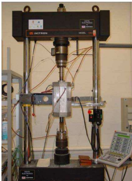
Figure 6 □ INSTRON 1362 fatigue machine [1].
