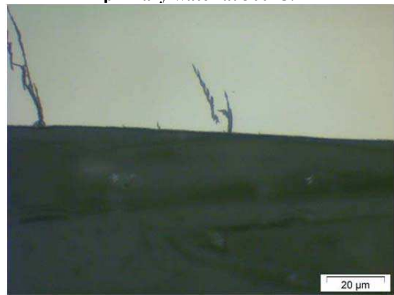
Figure 13 □ Cross section of 1630 MHI 11, \Delta\epsilon_t/2=0.5\% , \Delta\epsilon_t/dt=0.4\%/s , 10% cold rolled, PWR primary water at 300°C. Focus on initiation.
