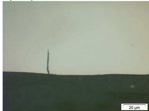
Figure 15 □ Cross section of 1630 MHI 14, \Delta\epsilon_t/2=0.5\% , \Delta\epsilon_t/dt=0.004\%/s , 10% cold rolled, PWR primary water at 300°C. Focus on initiation.
