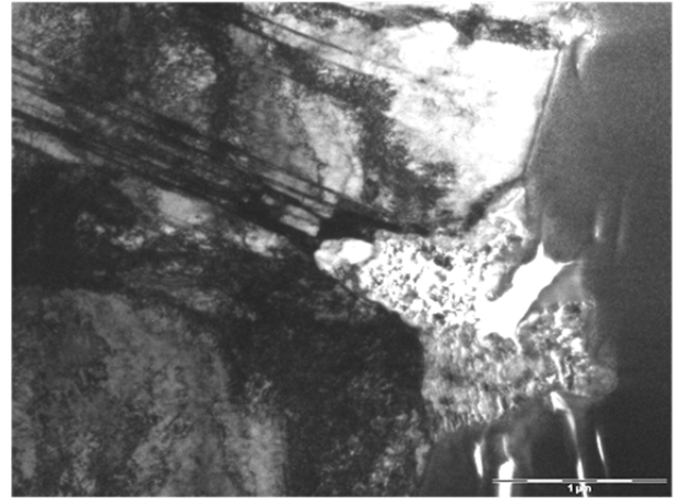
Figure 14 □Focus of crack initiation area as-received, \Delta\epsilon_f/2=0.5\% , \Delta\epsilon_f/dt=0.4\%/s 300°C, TEM BF, PWR primary water.
