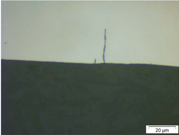
Figure 20 □ Cross section of 1630 MHI 04, \Delta\epsilon/2=0.5\% , 0.004\%/s , as-received 304L, PWR primary water at 300°C. Focus on initiation.
