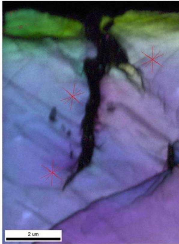
Figure 67 □ EBSD map of Cross section 1 of a TG crack on 1630MHIST7 with {110} plan traces, \Delta\varepsilon_t/dt=0.004\%/s , \Delta\varepsilon_t/2=0.5\% , 300cycles..
