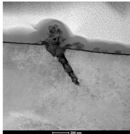
Figure 71 □ Cross section of crack initiation in 1630MHIST3, STEM HAADF, \Delta\epsilon_t/dt=0.4\%/s , \Delta\epsilon_t/2=0.5\% , 100 cycles.
