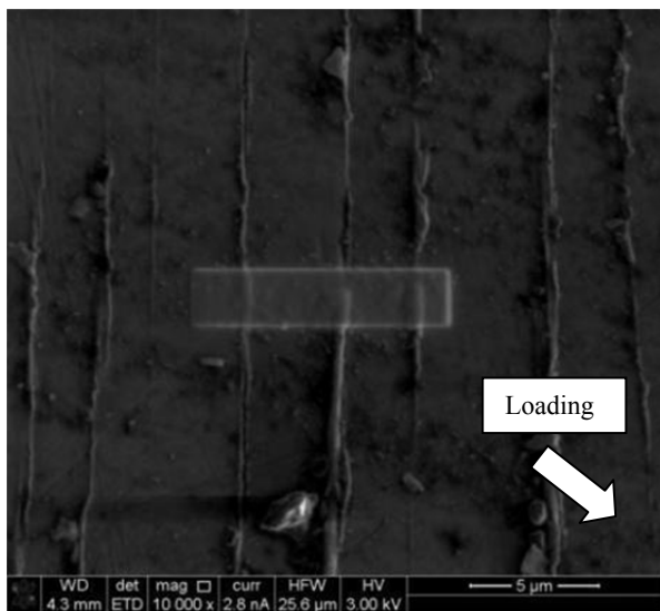
Figure 85 □ Fatigue crack initiation at the surface of sample 1630-78, \Delta\epsilon_t/2 = 0.5\% , \Delta\epsilon_t/dt = 0.4\%/s , 300°C.
