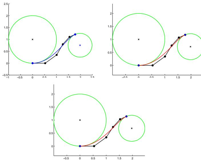
Figure 5.25: Control polygon for the S-shaped quintic PH spiral (left) and the S-shaped ATPH spirals with  $\alpha = \frac{7}{24}\pi$  (center),  $\alpha = \frac{5}{12}\pi$  (right) displayed in Figure 5.24.
