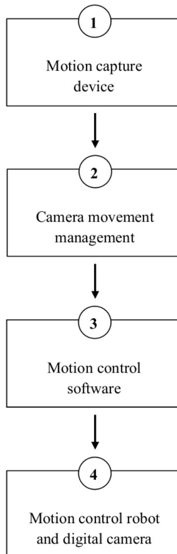
Figure 4.2: Motion control system diagram.
