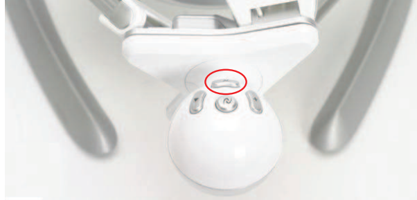
Figure A.2: In the red circle the back button on the Novint Falcon to record robot's positions.
