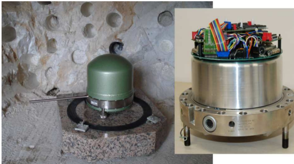
Figure 1.5: Integrated 3C broadband portable seismometer. Left side, STS-2 physically installed on a level surface, the instrument shows a rod oriented to the transverse direction, typically towards east geographic. Right side, a view of the internal part, where some electronic cards and a cylindrical package containing within three orthogonally oriented identical sensors.
