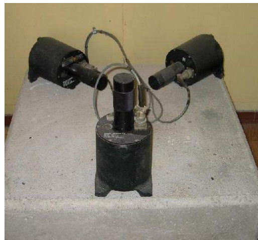
Figure 1.4: Short period single component seismometers designed for a 3C configuration, (one vertical Z and two horizontals X,Y).
