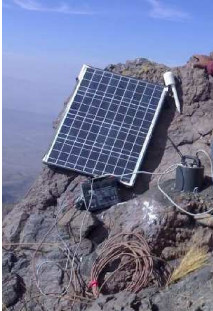
Figure 1.20: Photo of all components used for one seismic station. The seismometer 6TD is in the right middle with a Wi-Fi antenna. The white element lying in the corner of the solar panel is a GPS antenna, the blue square table is the solar panel and the black element below the solar panel is the battery.
