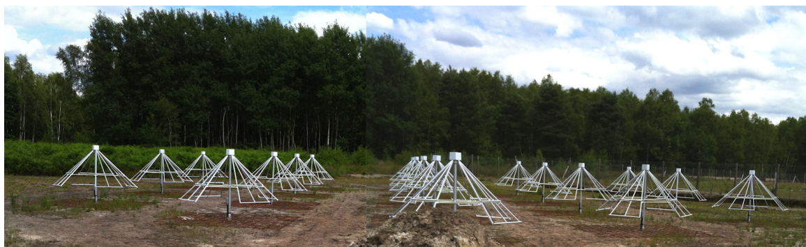
Fig. 4. The first LF tile prototype of the LSS built in Nançay in 2012, consisting of 19 crossed dipoles.
