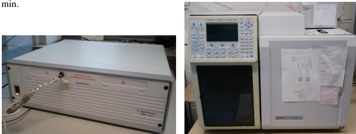
Figure 76. Chromatographie en phase gazeuse (g.) AGILENT 3000A (d.) VARIAN GC-3800.
