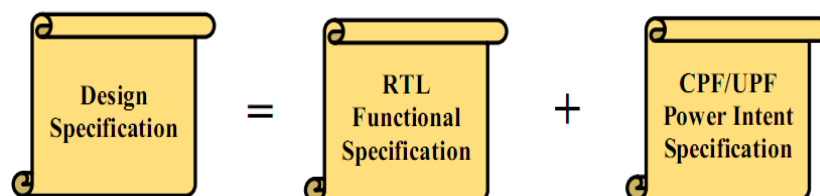
Figure 2.26: Functional and Power Intent
