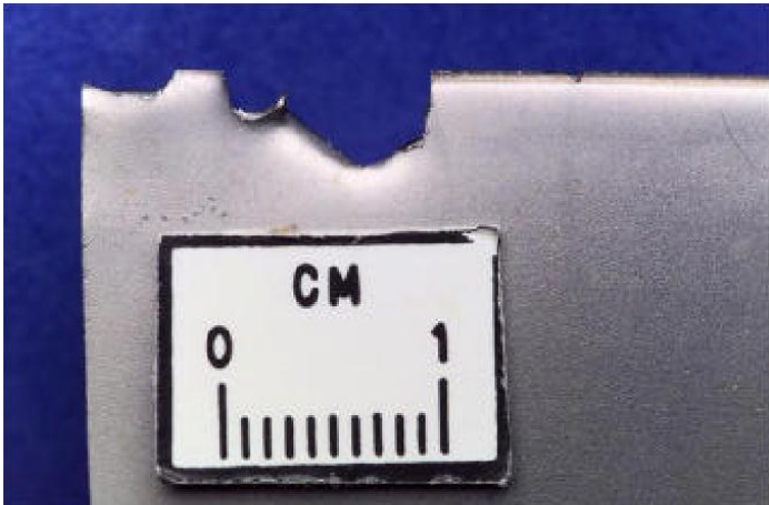
Figure 28 Blade damage due to surge (source: NASA)
