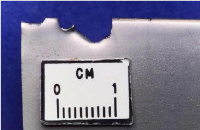
Figure 28 Blade damage due to surge (source: NASA)
