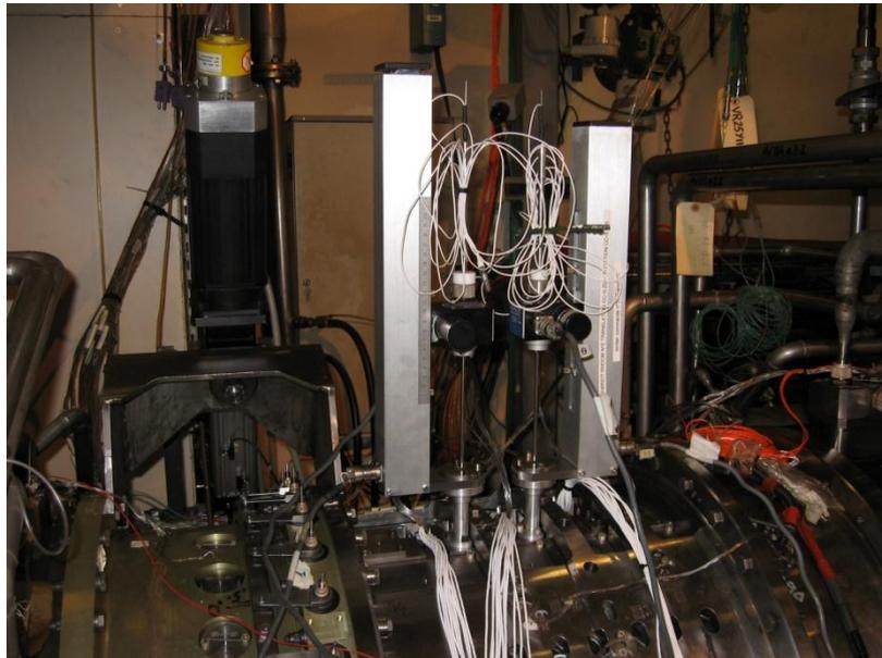
Figure 51 Experimental setup of the total pressure measurements
