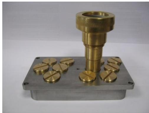
Figure 58 Removable block with a hopper extension mounted on the porthole
