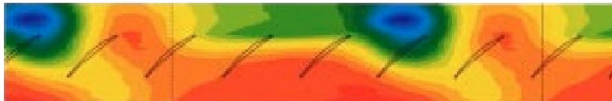
Figure 24 Pressure distribution over the rotor – visualization of the SLSD, (Inoue *et al.*, 2001, [41])
