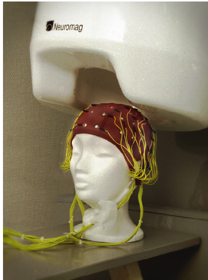
Figure 2.16 – Modern MEG device and a simultaneous EEG 64-electrode helmet.
