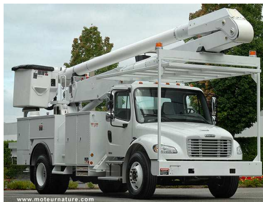
Figure 1.21 Camion hybride-parallèle de Freightliner aux Etats-Unis [Freightliner]
