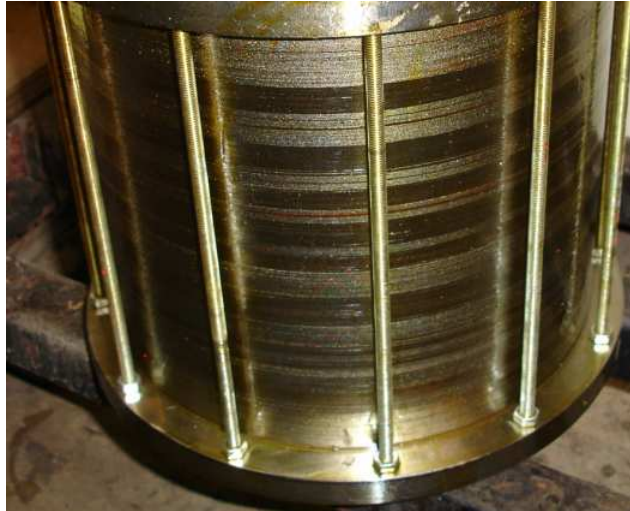
Figure 4.14 Tôles M270-35A de la machine prototype
