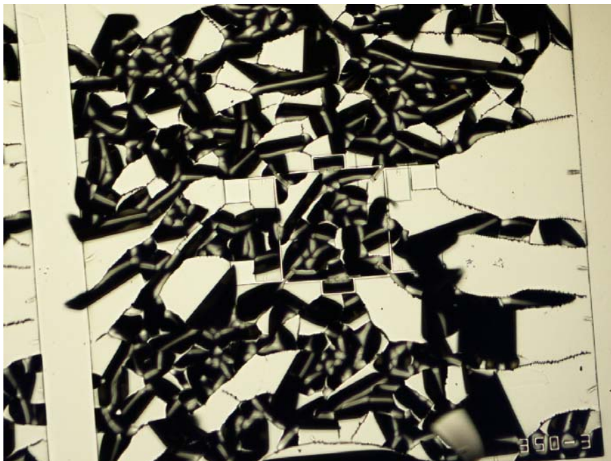
Figure 3.13: Metal peel-off due to large residual stress.
