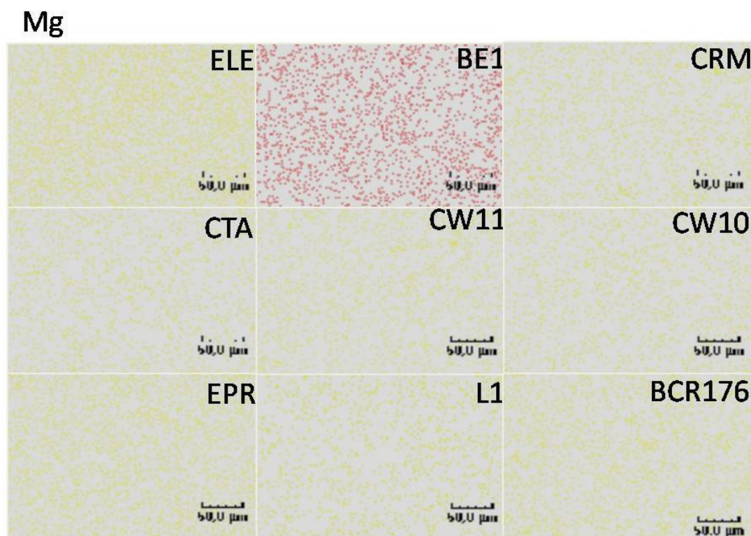
Figure III. 34: The SEM-EDS mapping on the pellets surface of magnesium presence in the samples.
