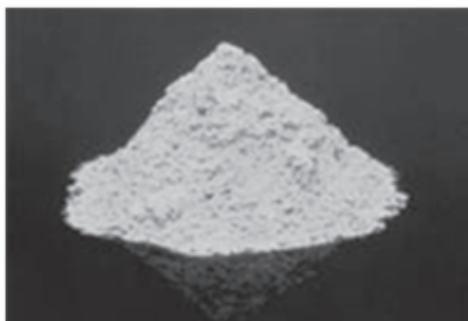
Figure I. 6: Fly ash is generally light tan in colour and consists mostly of silt-sized and clay-sized glassy spheres. This gives fly ash a consistency somewhat like talcum powder [12].
