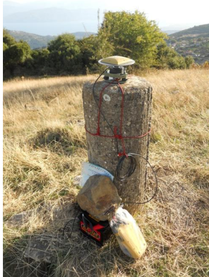
Figure 2-13. Placing the antenna over triblock and over pillar.
