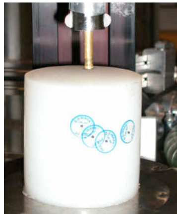
Figure 50: (Left) TC2 phantom undergoing torsional resonator testing at ETH Zurich. The phantom is made of Ecoflex 0030 (Smooth-On, Inc., Easton, PA) and includes randomly distributed Teflon beads embedded within it, rather than the regular grid of beads in the original Truth Cube.
