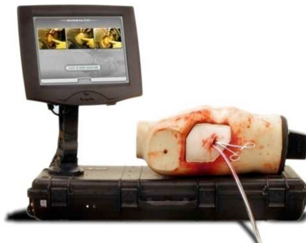
Figure 55: Prototype of the VIRGIL chest trauma training system. This version is the “classroom” version, another prototype was designed for use during military exercises. Both systems use tracking devices for the instruments, a touch screen for user interface navigation, and augmented reality to present the outcome of the training session.
