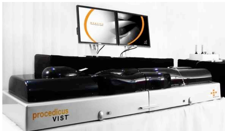
Figure 63: view of the complete VIST system for interventional radiology training. Although a major redesign of the hardware components was performed as well as improvements of the software, the core and the basic principles of the ICTS still apply.
