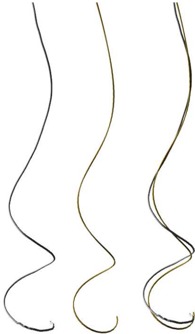
Figure 52: from left to right: reference coil model reconstructed from 3DRA data, simulated coil composed of 100 beam elements, and simulated model overlaid with actual data. The table on the right presents quantitative information about the difference between the simulated model and the real coil. This difference is very small even for large deformations.
