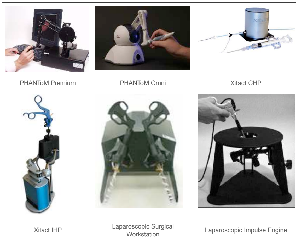
Figure 37: Some of the commercially available haptic devices frequently reported in the literature on medical simulation. Some of these systems are integrated in commercial simulators.
