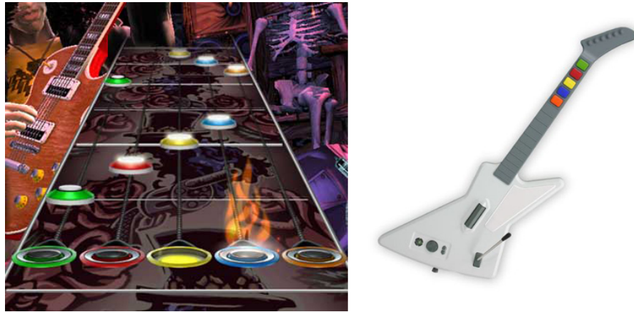
Figure 2: The Guitar Hero note chart and input device. While the note chart scrolls down, the non-dominant hand presses the fret button having the same color as the next note, and the dominant hand strums the strum bar when that note reaches the empty circles at the bottom of the screen. The visual feedforward and auditory feedback allows the player to perform complex bimanual multifinger rhythms with little practice (Activision Publishing)
