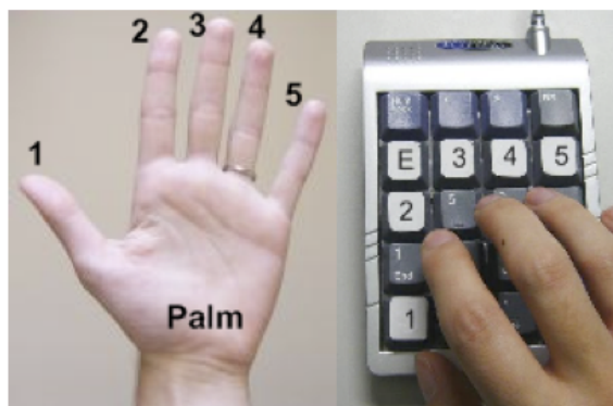
Figure 10: Five-key: A technique using sequences of short and long keypresses to enter any letter with just five keyboard keys (Szentgyorgyi and Lank, 2007)
