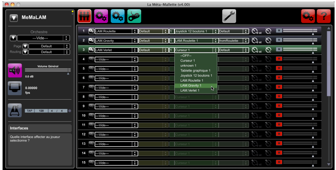
Figure 75: The user interface of the Metamallette for managing modules. The user selects the modules and mapping presets he wants to load in drop-down lists. He can manage to global parameters of the session on the left (load presets of whole configurations, set the main volume, etc.). And he can further edit the drivers of the input devices and the configuration of the synthesis engines by clicking on the colored buttons on the top.
