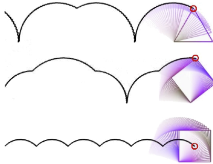
Figure 76: Roulette movements and resulting polygon motion
