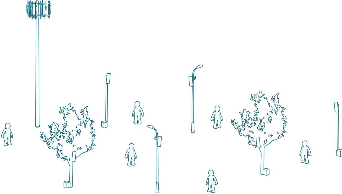
Figure 1.4: Typical small-cell deployment.
