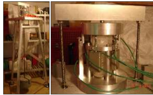
Figure 3. Testing device and salt sample below the upper plate.
