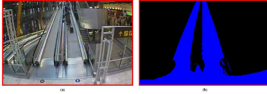
Figure 3.14: (a) Camera view. (b) Generated Region of Interest Image Map (RIIM) and blue region on the RIIM recommends Region of Interest Image (RII) .
