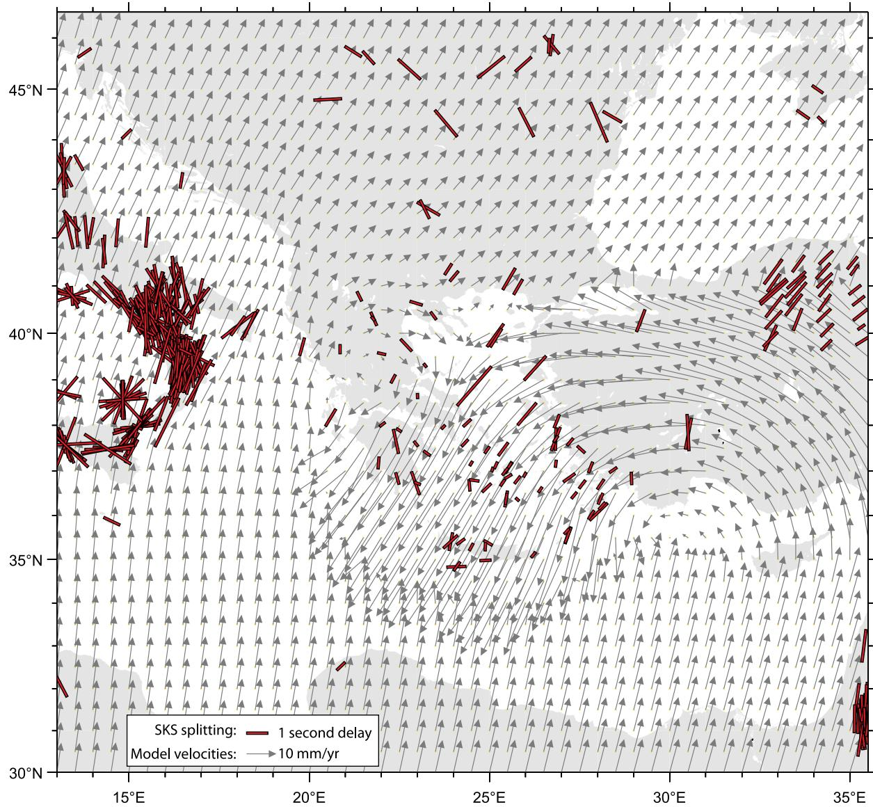
**Figure 12.** SKS splitting observations in Central and Eastern Mediterranean superimposed on our modeled Absolute Plate Motion. Shear wave splitting compilation is from Wüstefeld *et al.* [2009], database available online at <http://www.gm.univ-montp2.fr/splitting/DB/>.
