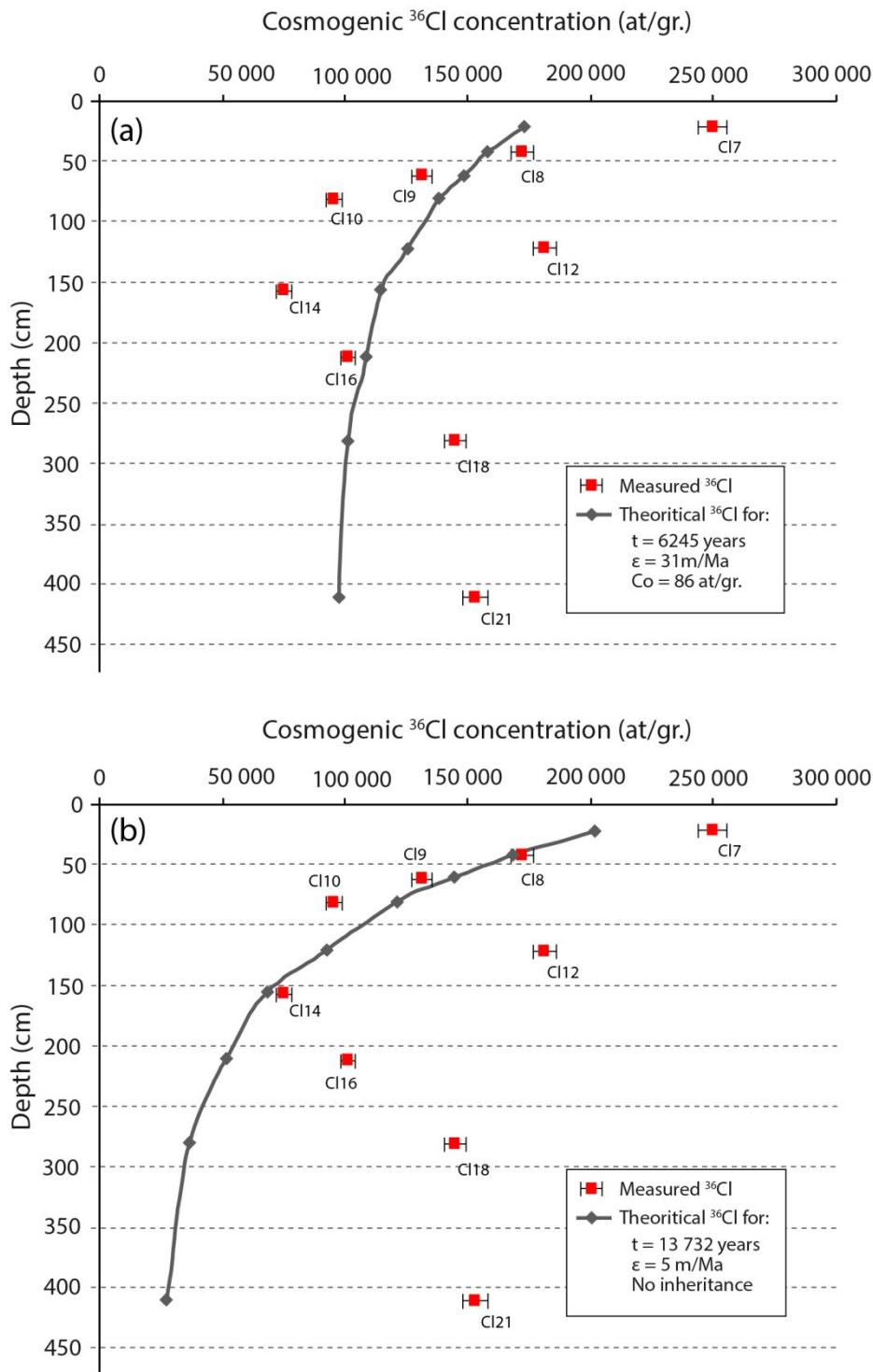
**Figure S8: Models of  $^{36}\text{Cl}$  concentrations for alluvial samples of the carbonate depth profile (historic colluviums are removed and then neglected, so that the 1.20 m depth is considered as the initial fan surface, see Figure S7).** (a) Model calculated on all samples; (b) Model excluding the three highest  $^{36}\text{Cl}$  concentrated samples (Cl12, Cl18 and Cl 21).
