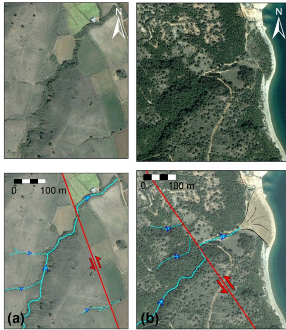
Figure S1: Possible offset streams along the southern Katouna fault.
