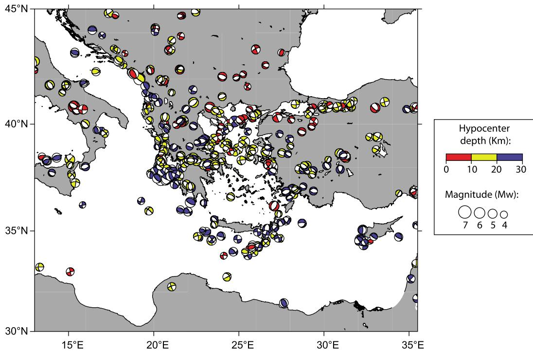
**Figure 3.** Input seismic moment tensors of the model. Fault plane solutions are from the Harvard CMT catalog (from 1976 to 2007) and the Regional Centroid Moment Tensor (RCMT) catalog (from 1995 to 2007). Location and hypocenter depth of the events are relocalized according to the *Engdahl et al.* [1998] catalog.
