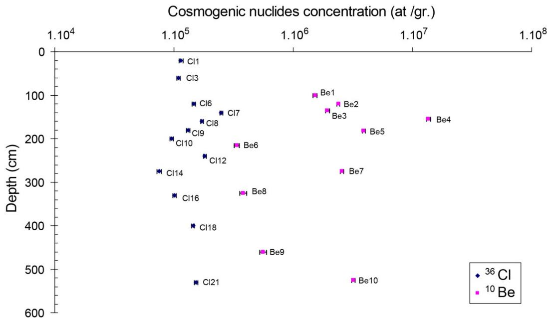
**Figure S5: Plot of measured  $^{36}\text{Cl}$  and  $^{10}\text{Be}$  concentrations as a function of depth (Values are in Table S1 and S3).**  $^{36}\text{Cl}$  and  $^{10}\text{Be}$  have been measured in carbonates and cherts, respectively. This plot emphasizes two distinct origins and exposure histories for carbonates and cherts.
