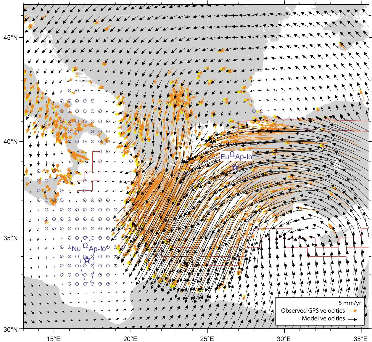
**Figure 8.** Observed and interpolated model velocities in the fixed Apulian-Ionian block reference frame defined in this study. Grid notches circled in blue have velocities  $<1$  mm/yr in this reference frame. Rotation pole of this Apulian-Ionian block relative to Eurasia ( $\text{Eu}^{\Omega}\text{Ap-Io}$ ) and to Nubia ( $\text{Nu}^{\Omega}\text{Ap-Io}$ ) are shown with their 95% confidence ellipse. Parameters of these Eulerian poles are given in Table 2.
