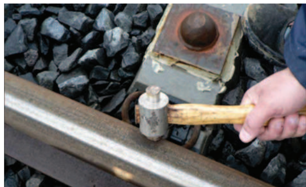
Figure 7.3 – receptance experience with the impact hammer: on-sleeper excitation [18]
